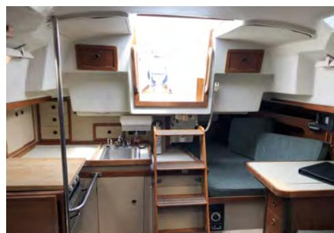
*Midnight Lady* is a fast, safe comfortable coastal cruiser. Below she is light and airy. The layout is fairly traditional with a V-Berth and head forward and a quarterberth aft. Port and starboard settees. The L-shaped galley next to the companionway makes for comfortable cooking.
